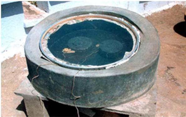
**Fig. 1: Cylindrical building material-housing solar cooker (BMHSC).**
