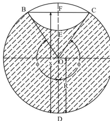
Fig. 6 Hatched portion shows the shadow area on the base plate for the condition  $\phi < 90^\circ$  and  $R < x$ .
