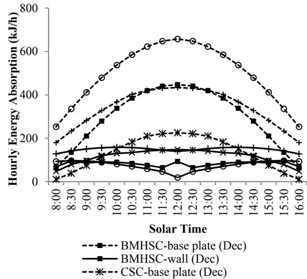
**Fig. 9** Variation in energy absorbed by the base plate and walls of the BMHSC and CSC with solar time for global radiation on Dec-21 and Jun-21.
