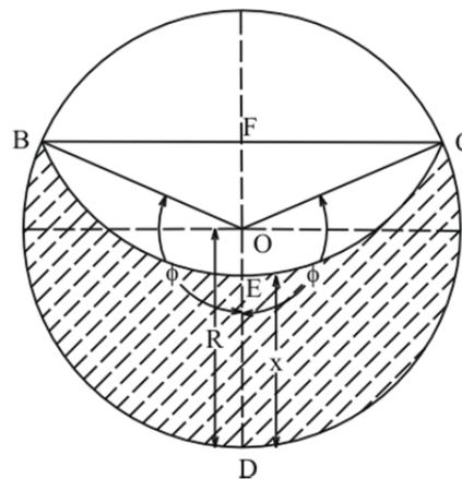
Fig. 5 Hatched portion shows the shadow area on the base plate for the condition  $\phi > 90^\circ$  and  $R > x$ .
