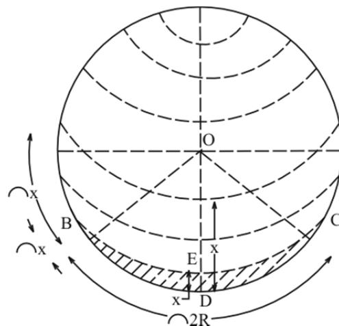
**Fig. 3 Shade length  $x$  on the absorber base plate. The dashed arcs represent the increase in shade with increase in angle of incidence of sunrays.**
