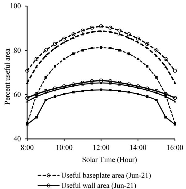
Fig. 7 Variation in useful base plate and wall areas of the BMHSC with solar time for three representative days of a year ( $\delta = -23.45^\circ, 0^\circ, 23.45^\circ$ )
