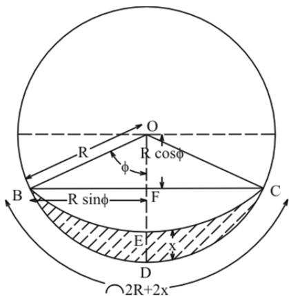
Fig. 4 Hatched portion shows the shadow area on the base plate for the condition  $\phi < 90^\circ$  and  $R > x$ .
