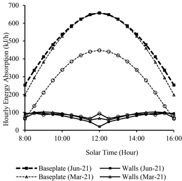
**Fig.8** Variation in energy absorbed by the base plate and walls of the BMHSC with solar time for global radiation on three different declinations ( $\delta$ ) of a year.
